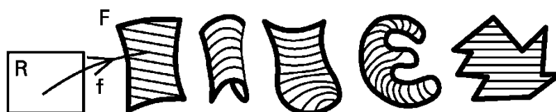
Figure 16: Examples of surface elements.
